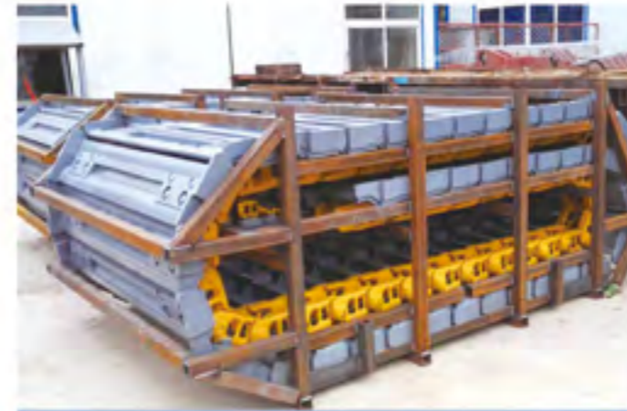
铆焊链板/ Weld Chain 宽度/ Width= 1.7m
