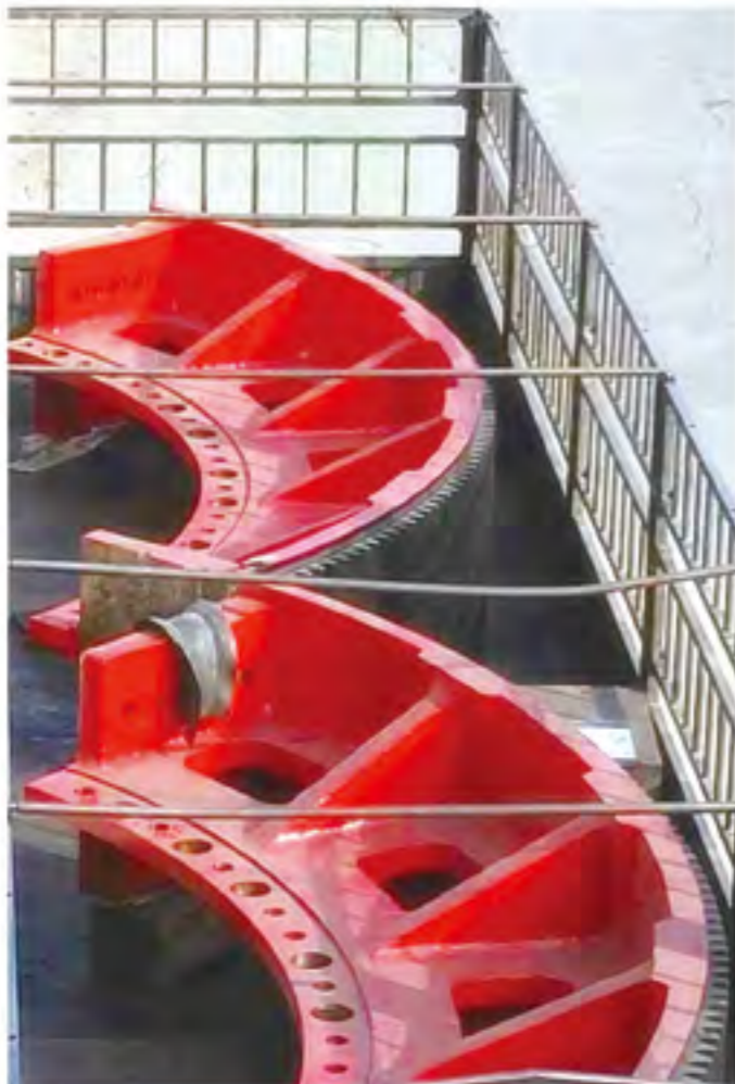
四分齿/ Girth Gear M=45 \phi =8.4m
