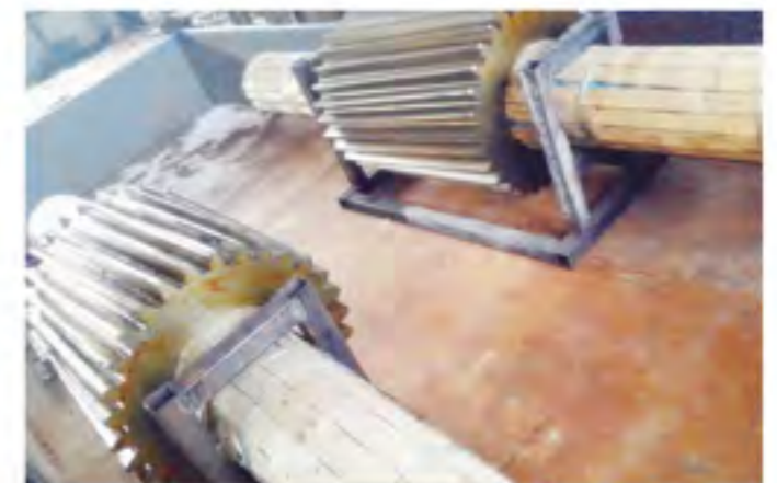
齿轴/ Gear Shaft L=3.4m
