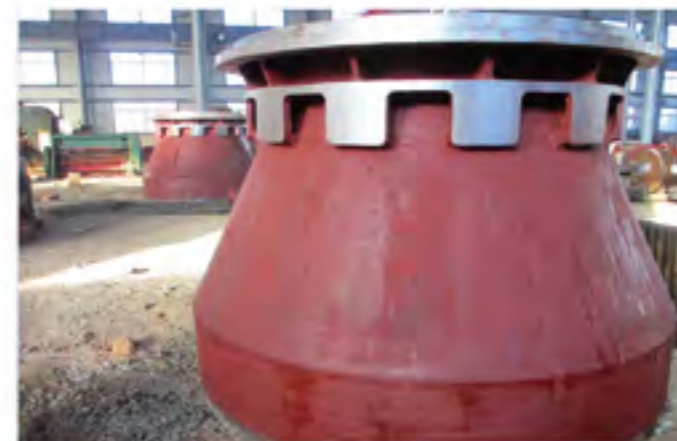
回转窑出料口/ Outlet of Rotary Kiln
