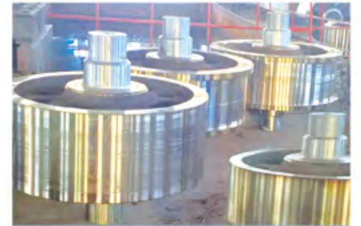
托轮/ Riding Wheel \phi=1.5m
