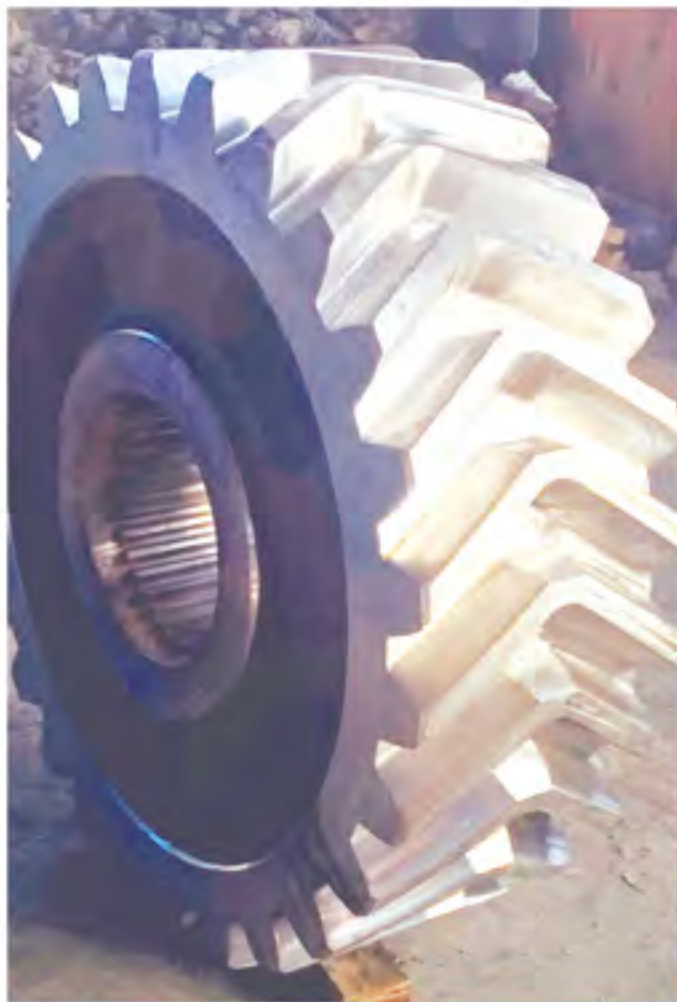
电炉人字齿/ Double Helical Tooth M=36 \phi=1.4m
