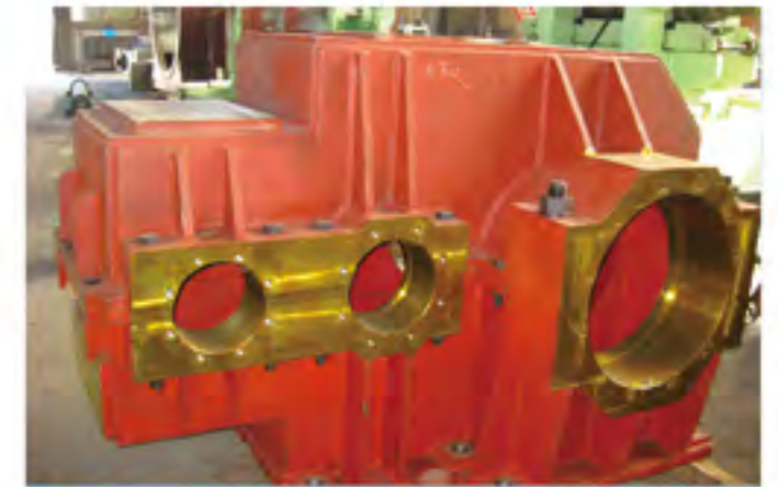
减速机箱体/ Gear Reducer Box H=1.8m L=3m
