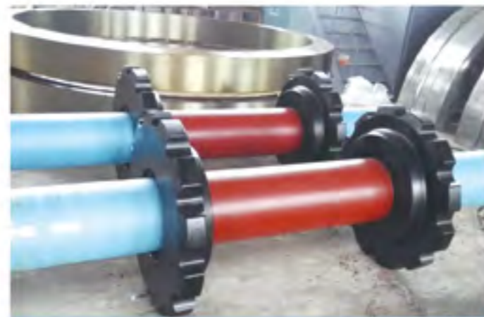
链轮/ Chain Wheel \phi=1.1m
