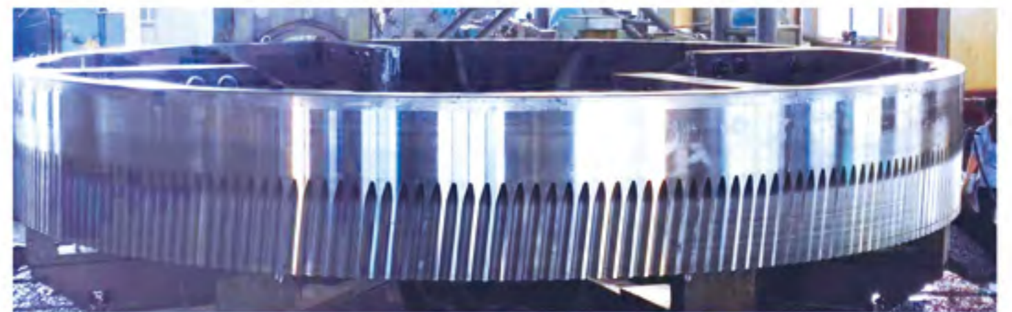
齿圈/ Girth Gear M=20 \phi=6.4m
